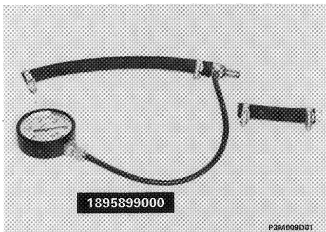
Vacuum gauge with connections for checking, on the car, the efficiency of the vane-type vacuum units
