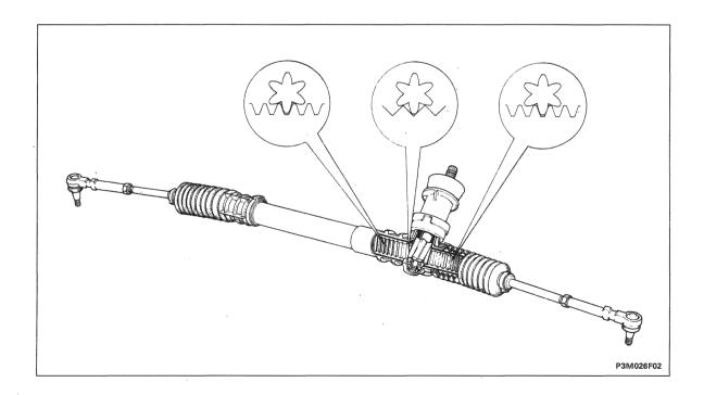
View of the variable-ratio steering gear with schematic representation of the rack teeth and pinion.
